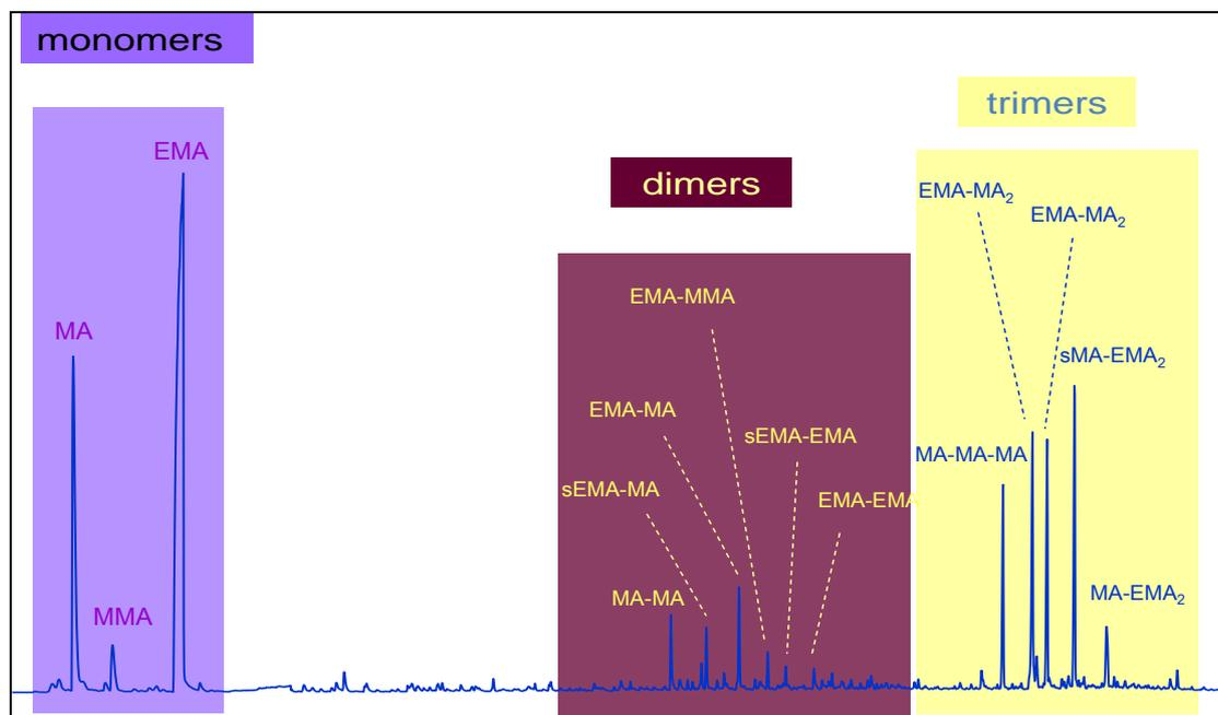
Figure 40: Pyrogram of Paraloid B72 at 600°C.
