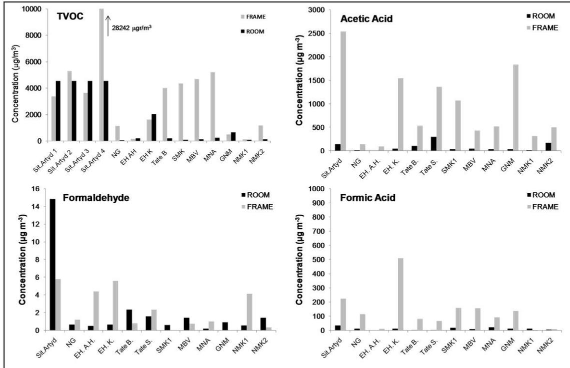
Figure 19: Total concentration of volatile organic compounds (TVOC), acetic acid, formic acid and formaldehyde measured inside and outside microclimate frames. For location abbreviations see Table 3 and table in Figure text 12.
