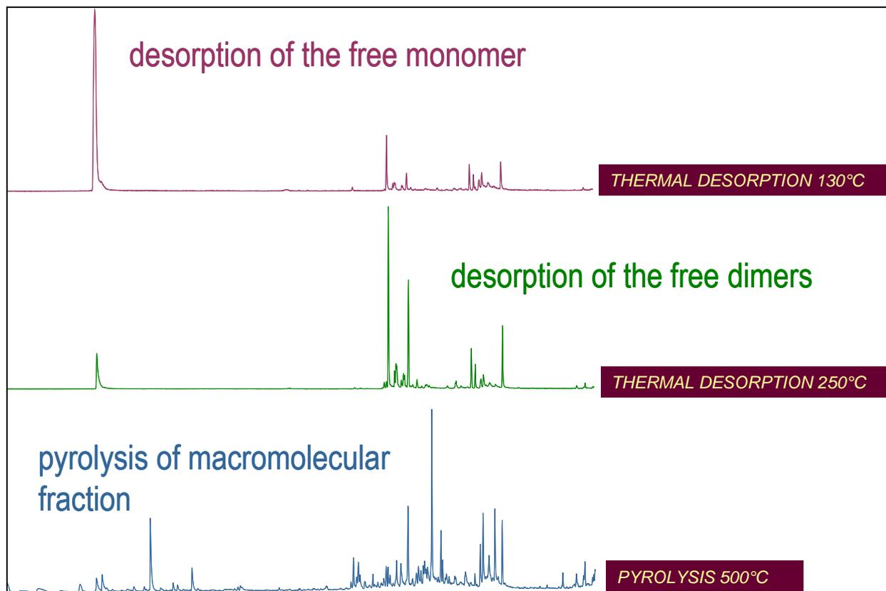
Figure 42: GC-MS chromatograms of raw MS2A exposed at 130 °C, 250 °C and 500 °C.
