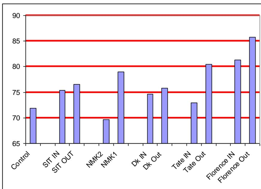
Figure 52: Graph shows the plot of  $T_g$  (°C) vs. sites. IN = Inside microclimate frames. OUT = outside microclimate frames.
