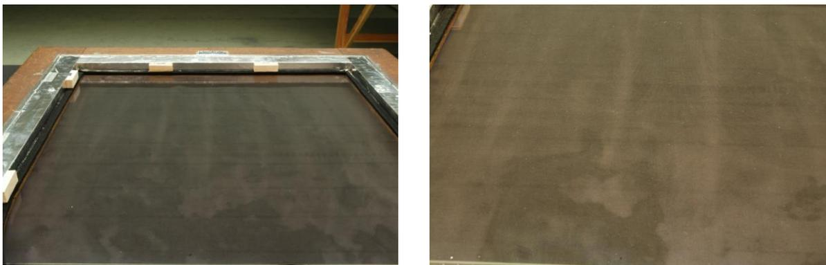
Fig. 4. Whitish deposits on inside of glass of the microclimate box, photographed (on a black cloth), 11 July 2007.
