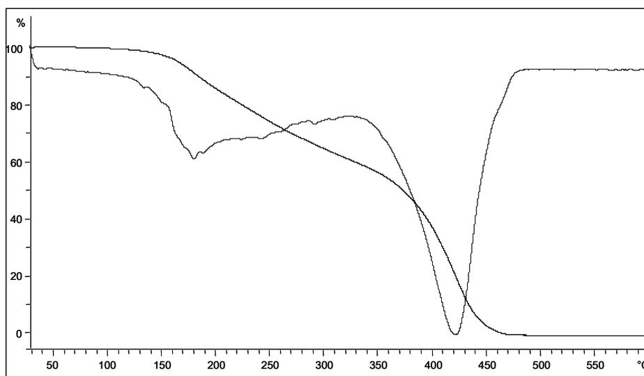
Figure 41: Thermogravimetric graph for MS2A (continuous line) and relative derivative (dashed line).
