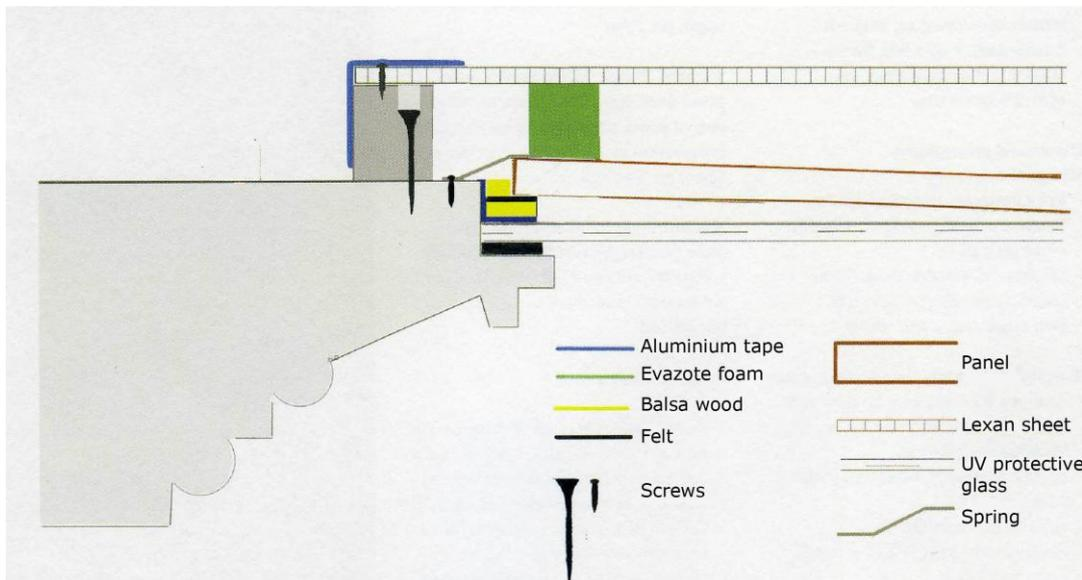
Fig. 1. Diagram showing cross-section of the construction of microclimate boxes used in the Mauritshuis.
